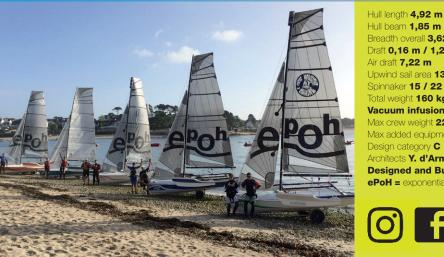
Hull beam 1,85 m Breadth overall **3,62 m** (2,03 m stored) Draft 0,16 m / 1,20 m Air draft 7,22 m Upwind sail area 13 / 16 m<sup>2</sup> Spinnaker 15 / 22 m<sup>2</sup> Total weight **160 kg** (143 kg without floats) Vacuum infusion sandwich technology Max crew weight 225 kg Max added equipment weight 30 kg Design category **C** (ICNN certified)
